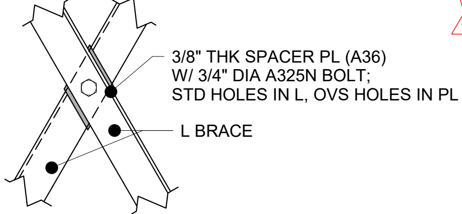
13 BRACE X CONNEX PLAN 1 1/2" = 1'-0"
